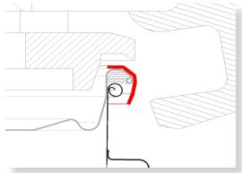
In the first stage, the lid including clamping ring will be placed on the fuselage.
